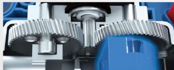
double gears drive the balancing block
